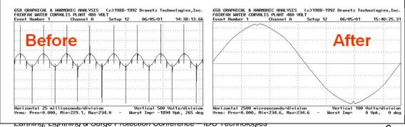
The effective elimination of low level oscillatory transient events occurring inside the envelope of the sine wave is one of the most beneficial and immediate methods of obtaining significant reduction of system lock-ups and unnecessary resets – thus leading to much more immediate return on investment and the optimal protection of high speed microprocessor based systems, e.g. PLC's, timing controls, robotic control systems, RTU's, Variable Frequency Drives etc.
