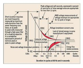
The most oft quoted standard is the CBEMA curve. From "Understanding the CBEMA Curve (www.marcspages.co.uk): " To simplify matters the Computer and Business Equipment Manufacturers Association came up with a curve wherein the voltage deviation from the norm is the only factor taken into account. It is felt that equipment fitted with a filter should be able to withstand greater deviations the shorter the timing of the deviation.
