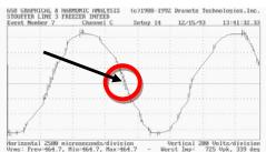
circle. This event expanded in the following figure illustrates what in fact amounts to nine "false" zero crossings of the sine wave. These graphs were from a processing facility in 1993. These events caused random lockups and shut downs of the line resulting in the loss of tens of thousands of dollars in products.
