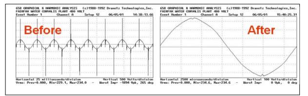
The effective elimination of low level oscillatory transient events occurring inside the envelope of the sine wave is one of the most beneficial and immediate methods of obtaining significant reduction of system lock-ups and unnecessary resets – thus leading to much more immediate return on investment and the optimal protection of Smart Meters, SCADA systems, Substation Reclosers, PhotoVoltaic invertors and all other high speed microprocessor based systems.
