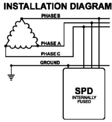
When inspecting the panel for installation, make a visual check that there are no Neutral to Ground bonds that violate the NEC/CEC. <sup>†</sup>[ex.: NEC '10-foot tap rule' for direct bus tapping.].
