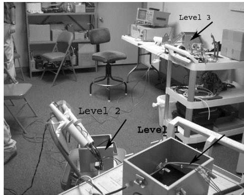
However when applying that same test impulse to the technology referenced as frequency-attenuating, the difference was over 900 volts between Unit 1 and the residual voltage measured at Unit 2.
