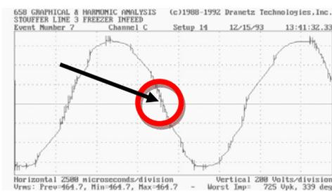
This event expanded in the following figure illustrates what in fact amounts to nine “false” zero crossings of the sine wave. These graphs were from a processing facility in 1993. These events caused random lockups and shut downs of the line resulting in the loss of tens of thousands of dollars in products.
