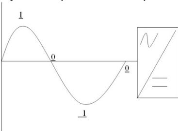
However, due to the presence of SCR/VFD created ringing transients we may quickly arrive at the supposition that when the 0 crossings are distorted due to the presence of these events, a series of false zero crossings are created; thus
