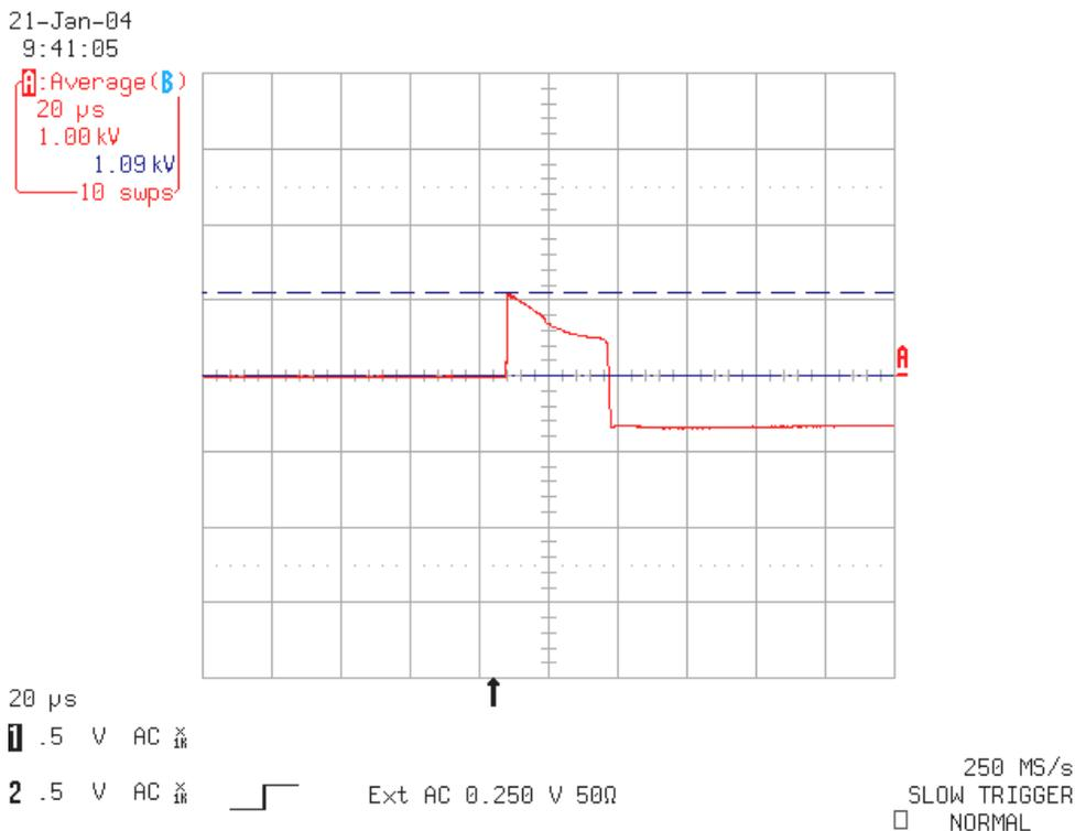
I then cut the leads to remove 5.5 inches from both the Line 1 and Neutral leads. This reduced the lead length from the board to the end of the lead to 18 inches. The let through voltage recorded for the unit after application of the B3/C1 test wave was 960Vpk. The image from the scope is shown below:
